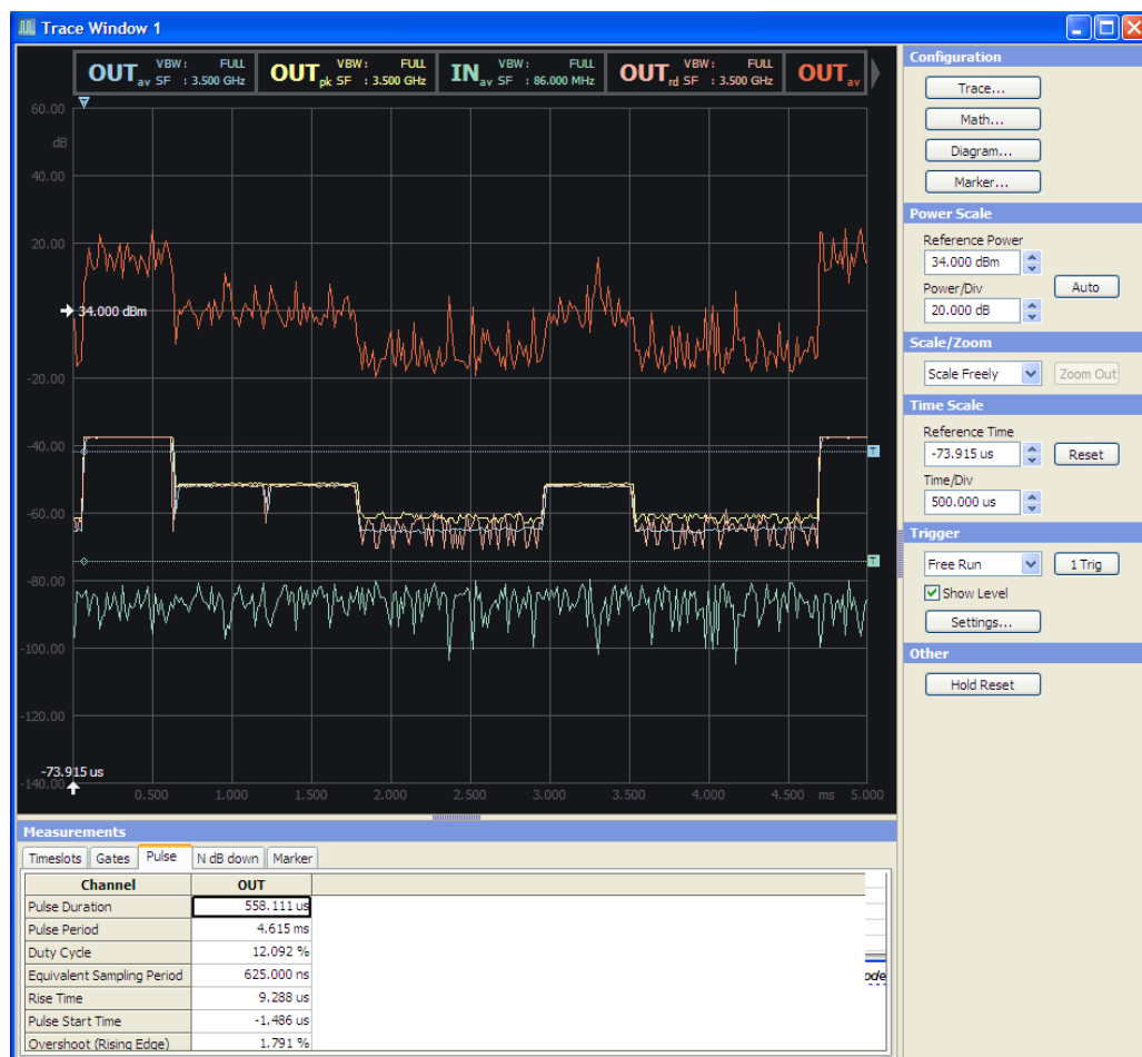
Figure 4-12: Operating concept > Numerical measurement window
