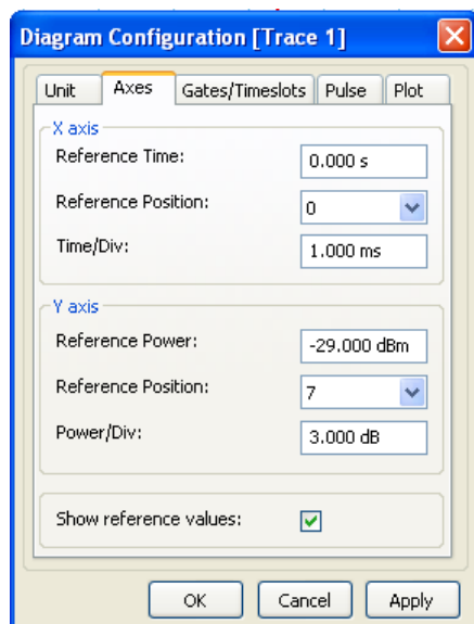
Figure 5-37: Measure > Trace > Diagram > Axes
