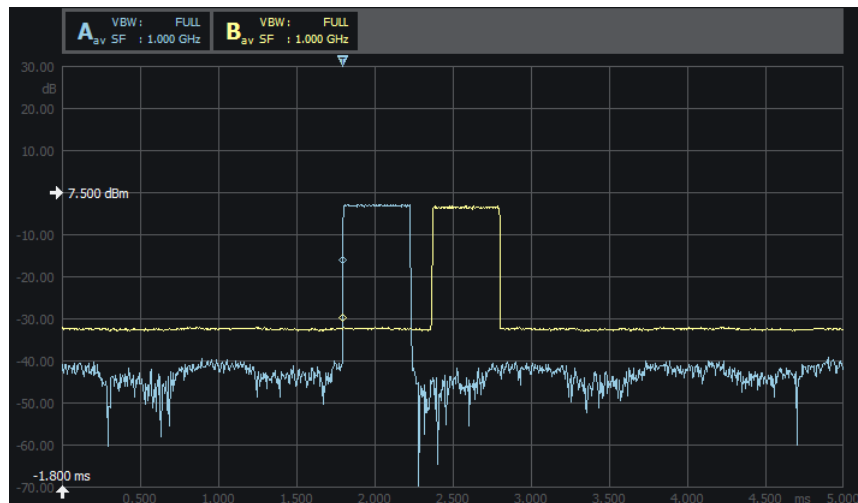
Figure 5-42: Marker example > two traces carrying pulses
